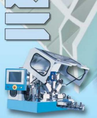
A 'HIGHFLOW' VERSION OF THE ECOLINE PREPPING CENTRE WITH DEDICATED TOOLING HEADS FOR HIGHER OUTPUT WHERE FLEXIBILITY IS NOT REQUIRED.
