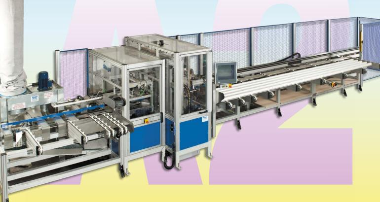
THE AUTOFLOW 2 IS DESIGNED FOR ALL CASEMENT WINDOWS, TILT AND TURN, VERTICAL SLIDERS, ALL DOORS INCLUDING BI FOLDS, RESIDENTIAL DOORS, FRENCH DOORS AND INLINE SLIDERS PRODUCING AN OUTPUT OF APPROXIMATELY 400 WINDOWS PER WEEK.
