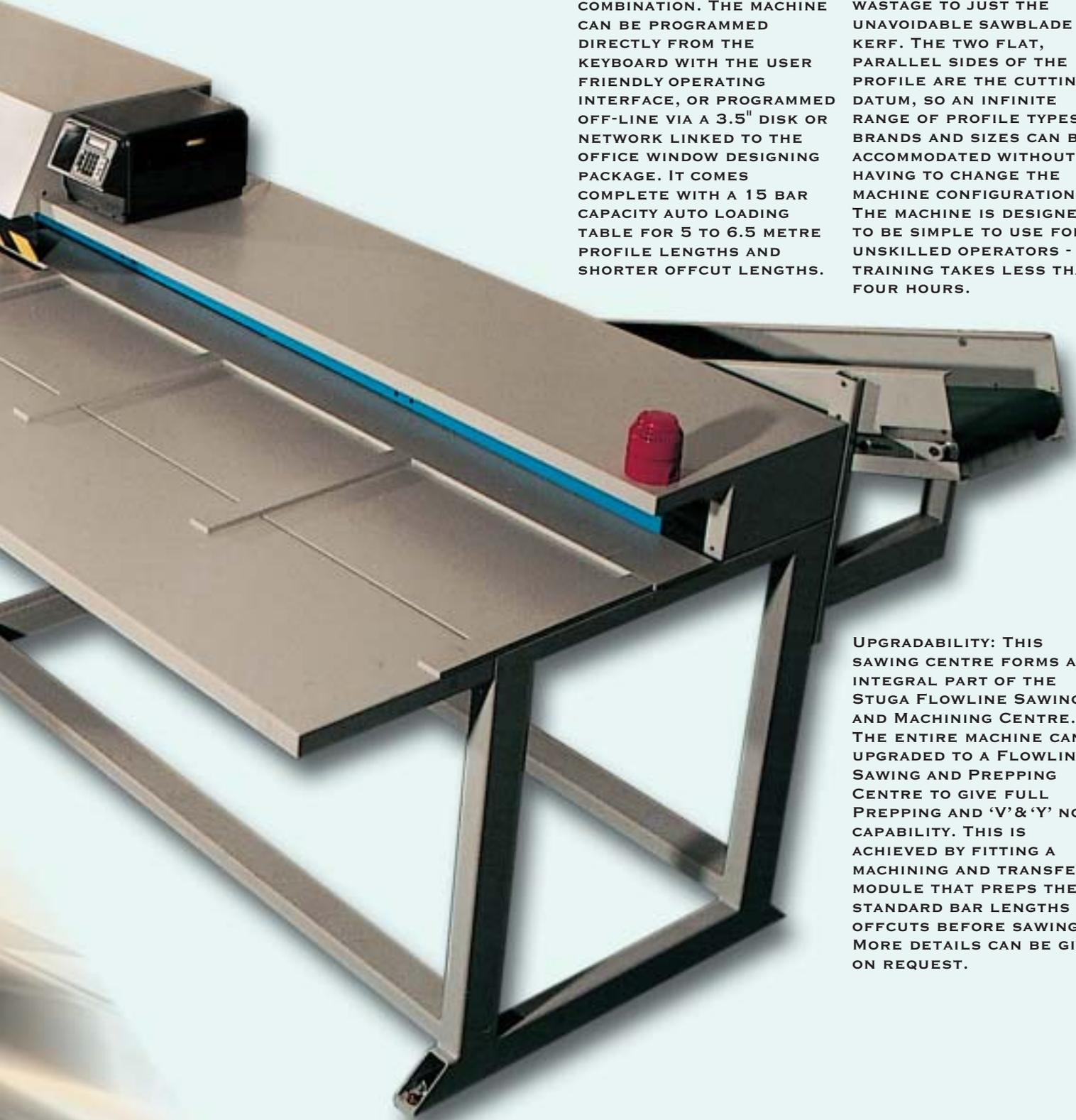
**UPGRADABILITY:** THIS SAWING CENTRE FORMS AN INTEGRAL PART OF THE STUGA FLOWLINE SAWING AND MACHINING CENTRE. THE ENTIRE MACHINE CAN BE UPGRADED TO A FLOWLINE SAWING AND PREPPING CENTRE TO GIVE FULL PREPPING AND 'V' & 'Y' NOTCH CAPABILITY. THIS IS ACHIEVED BY FITTING A MACHINING AND TRANSFER MODULE THAT PREPS THE STANDARD BAR LENGTHS AND OFFCUTS BEFORE SAWING. MORE DETAILS CAN BE GIVEN ON REQUEST.
